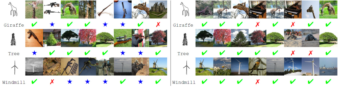
Figure 5.1: Left hand column shows the top-8 retrieval instances for a few sketch queries from the Sketchy dataset using \mathcal{L}_{\text{semantic}} + \mathcal{L}_{\text{triplet}} + \mathcal{L}_1 model. The green checks denote correctly retrieved classes, while the red crosses denote images from incorrect class. The blue stars denote the hub instances occurring repeatedly from a particular common class for most of the classes ( rifle in this case). The right hand column shows the top-8 retrieval images for the same query sample using the full model. Notice that there are no hub instances generated here.
